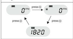
It will return to detection interface after no operation for 6 seconds.
