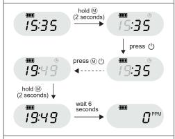
During the processing, it will return to detection interface after no operation for 2 minutes.
